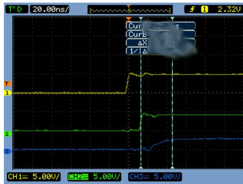
Messung des Propagation Delays, Kanal 1:  $D_{in}$ , Kanal 2: Clock, Kanal 3:  $D_{out}$ .
